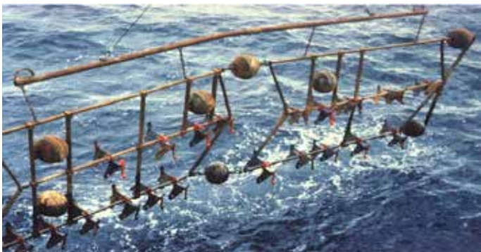
The plough-harrow apparatus used to disturb the seafloor in 1989. During this experiment, nodules were not recovered but ploughed into the sediment.
