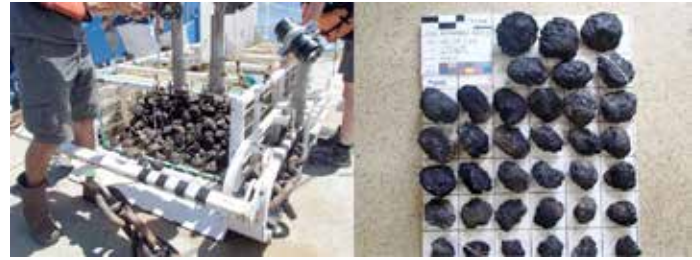
Figure 3: The dredge (left) and a size-sorted sample of nodules (right) obtained during cruise GSRNOD14A.
