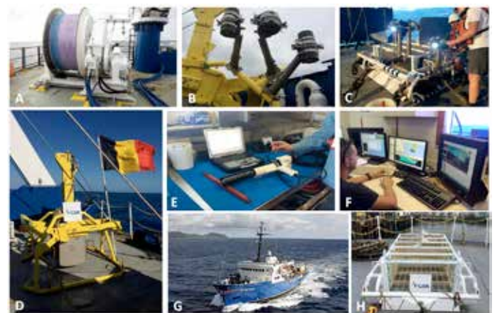
Figure 2: Vessel and equipment used during GSRNOD14A: (A) Winch used for sampling, (B) camera equipment mounted on box-corer, (C) camera equipment mounted on dredge, (D) 50x50x50cm box-corer, (E) Sippican and launching system, (F) MBES acquisition, (G) R/V Mt. Mitchell and (H) dredge.
