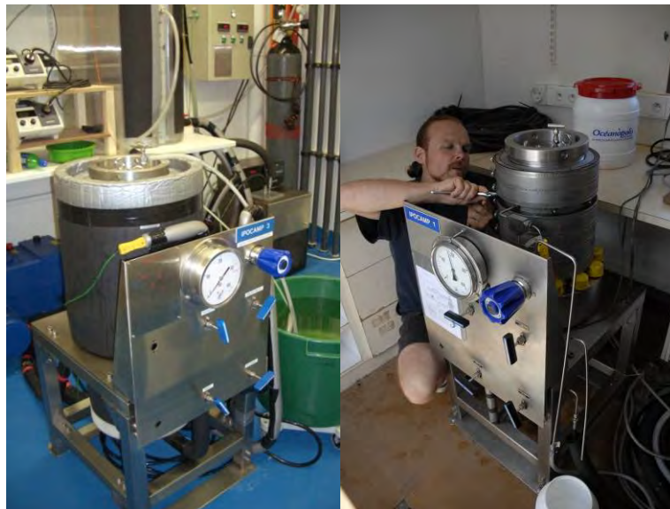
Figure 5: The IPOCAMP pressure aquarium. Left: IPOCAMP #3, in service at the National Oceanography Centre (Partner 5). Right: IPOCAMP #1 (Partner 25), mounted onboard R/V "Pourquoi Pas?" (Ifremer) during a MoMAR cruise in 2012.
