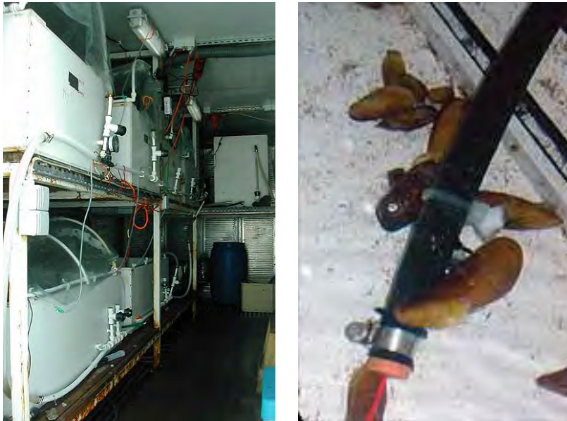
Figure 3: The LabHorta facilities for live maintenance of vent mussels B. azoricus (from http://www.horta.uac.pt/projectos/fisiovent/labhorta.htm )
